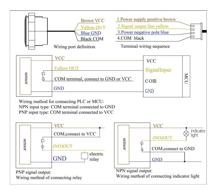
Working principle of relay NC point output:
