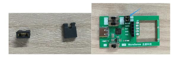
3.For IO adjusting parameter, optional 4 distance level, you could switch the bottom as green square and arrow area.left is "0", right is "1" (digital signal)
