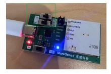
2.For UART adjusting parameter, the 2pcs jumper need to be added in the testing board as blue arrow marks showing location.
