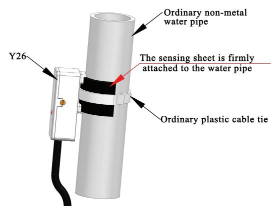
The height of the sensed liquid level is related to the sensitivity of the sensor. The higher the sensitivity, the lower the sensed liquid level
