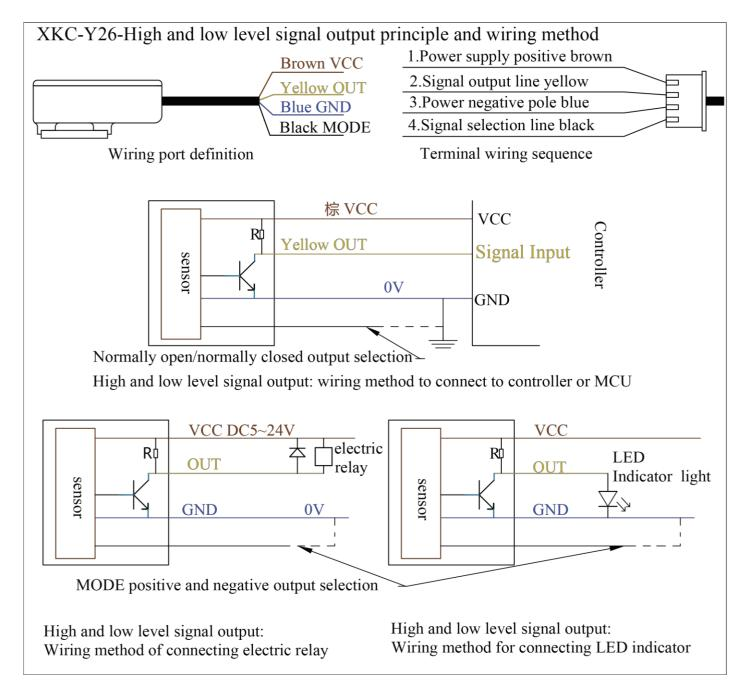
High and low level output drive small electric relay (coil current ≤100mA) Product Applications:
