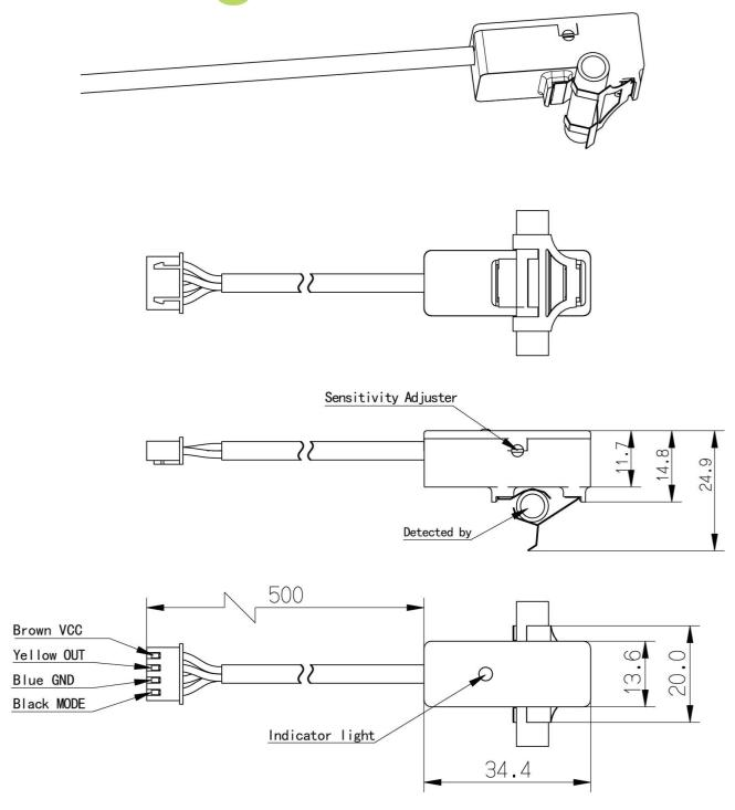
9th.Y26A wiring diagram of various models
