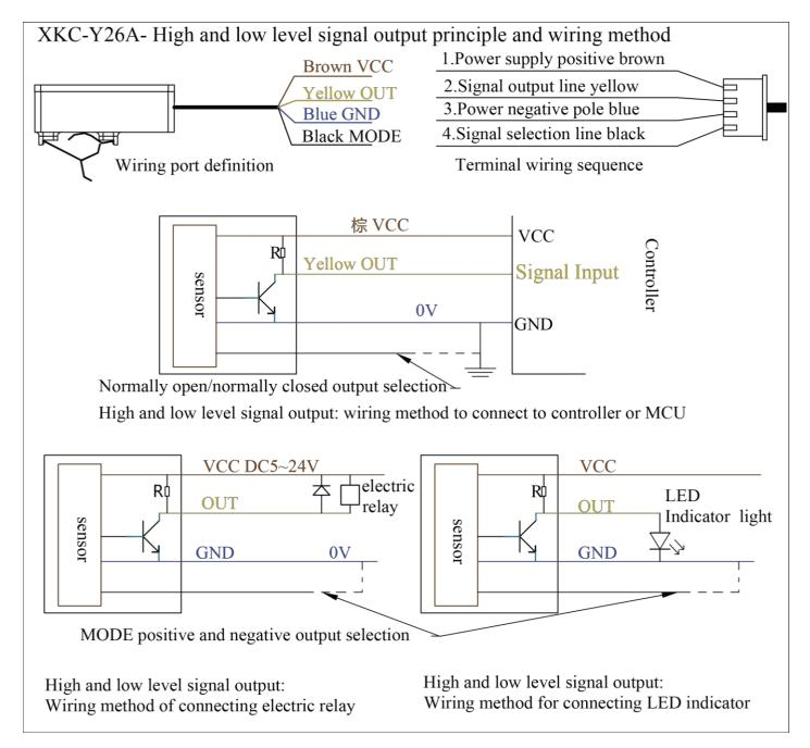
High and low level output drive small electric relay (coil current ≤100mA) Product Applications:
