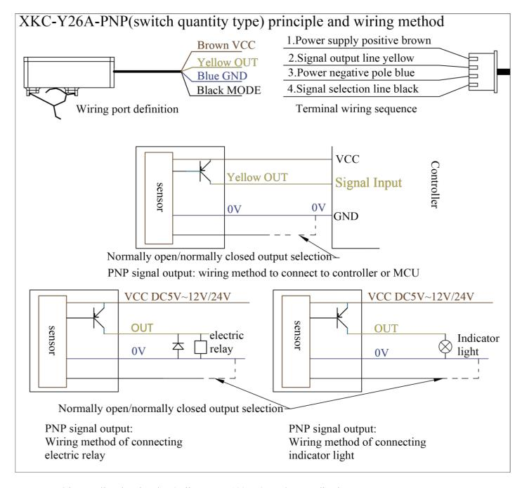
PNP output drive small electric relay (coil current ≤100mA) Product Applications:
