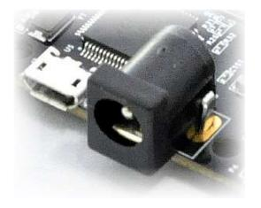
connecting the power supply. Please refer to the marking on the board for more details. The external power supply should be in the range of +5 to +12V, with sufficient current rating.
