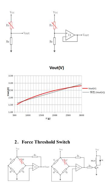
This is an ideal circuit for applications that require on-off switching at a specified force. It consists a Wheatstone bridge circuit and a voltage comparator.
