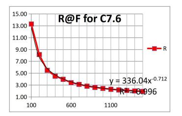
The following plot shows an near-linear curve which is 1/R @F.
