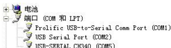
2. Connect only one device and power on separately. Click the test baud rate of the software. The software will test the baud rate and address of the current device. The default baud rate is 4800 bit/s and the default address is 0x01.
