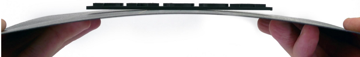
Pict. 13 - Removing the model from the PEI print surface by bending the steel sheet.
