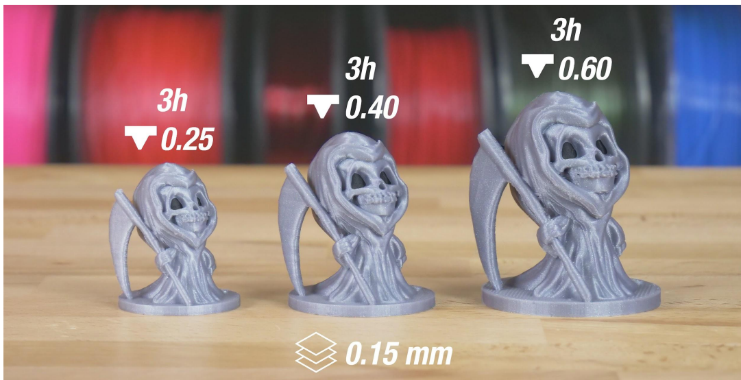
Pict. 22 - Different nozzle sizes have big impact on print speed
