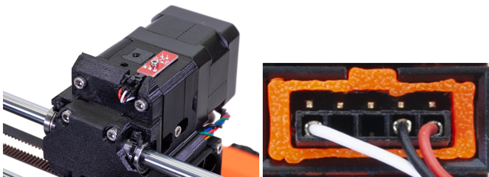
Pict. 38 - Properly connected and seated filament sensor
