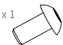
18 Hexagon socket flat round head screw M5X8 x 6 内六角平圆头螺钉M5X8
