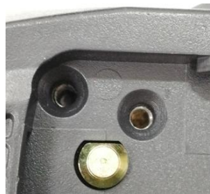
6.Fix the mechanical lock to the case by 2 M5*10 flat head cross screw
